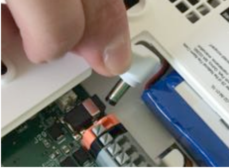
Plug in the power connector
