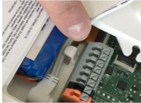
Route the wire behind the retainer clip
