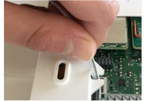
Insert the wire into the strain-relief
