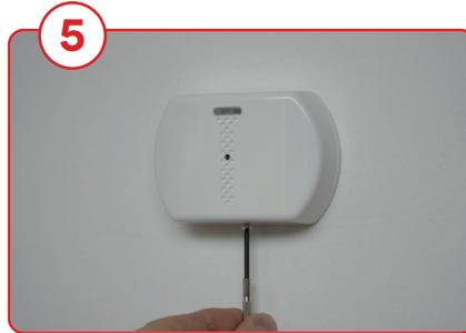
5 Use the tiny screw that is included to secure the cover to the backplate on the bottom of the device.
